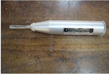
Alat Uji Pantul Beton
